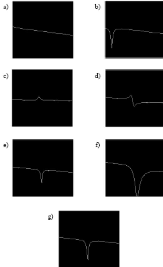
3. Tune the signal phase. Adjust the Frequency and Signal Phase until the dip is in the center and the depth of the dip is maximized and symmetric.
